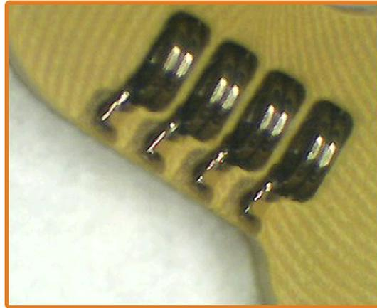
*Figure 2: Snap In Contact Sets With No Beams or Elastomers*
