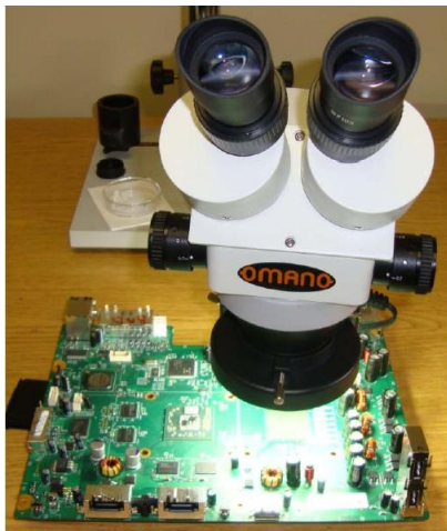
Figure 4: Examining the board under a stereomicroscope.
