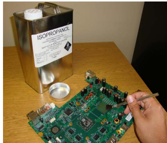
Figure 5: Cleaning the board pads with alcohol and brush.
