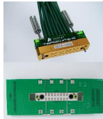
Diagram 1: TR40-SM-8X1 showing board and dowel pins keyed for mating.
