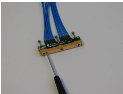
Figure 1: Removing the M1 Screws
