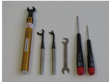
Figure 1: Recommended Permissible Hardware Instruments
