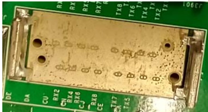
Figure 7: Example of resin on footprint after reflow. It is recommended to remove the residue with the appropriate cleaner to prevent connection problems.
